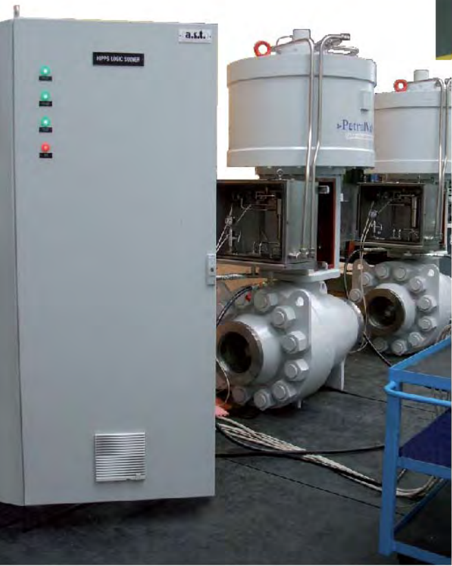
HIPPS VALVES, ACTUATORS, CONTROL SYSTEMS, LOGIC SOLVER - INTEGRATED FUNCTIONAL TEST (I-FAT)
